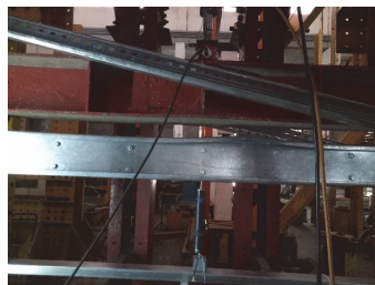
FIGURE 11. Crushing failure on the beam's top flange
