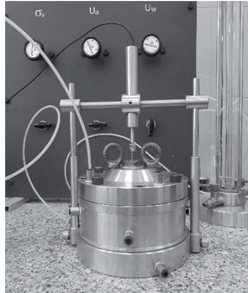
FIGURE 5. Consolidometer used in tests
