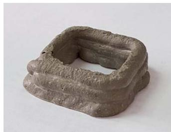
FIGURE 6. Mortar test in 3D printing
