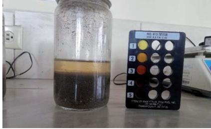
FIGURE 2. Collation through a color plate for the analysis of organic matter content in the fine aggregate
