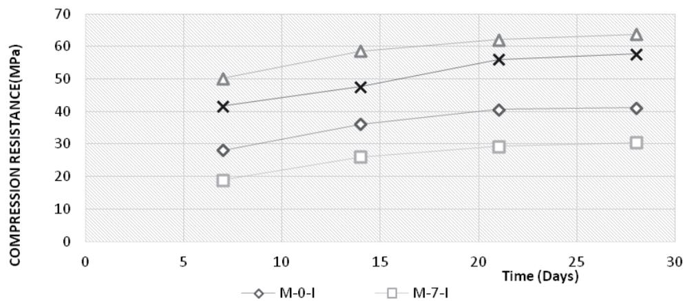
FIGURE 5. Evolution of long-term compressive strength
