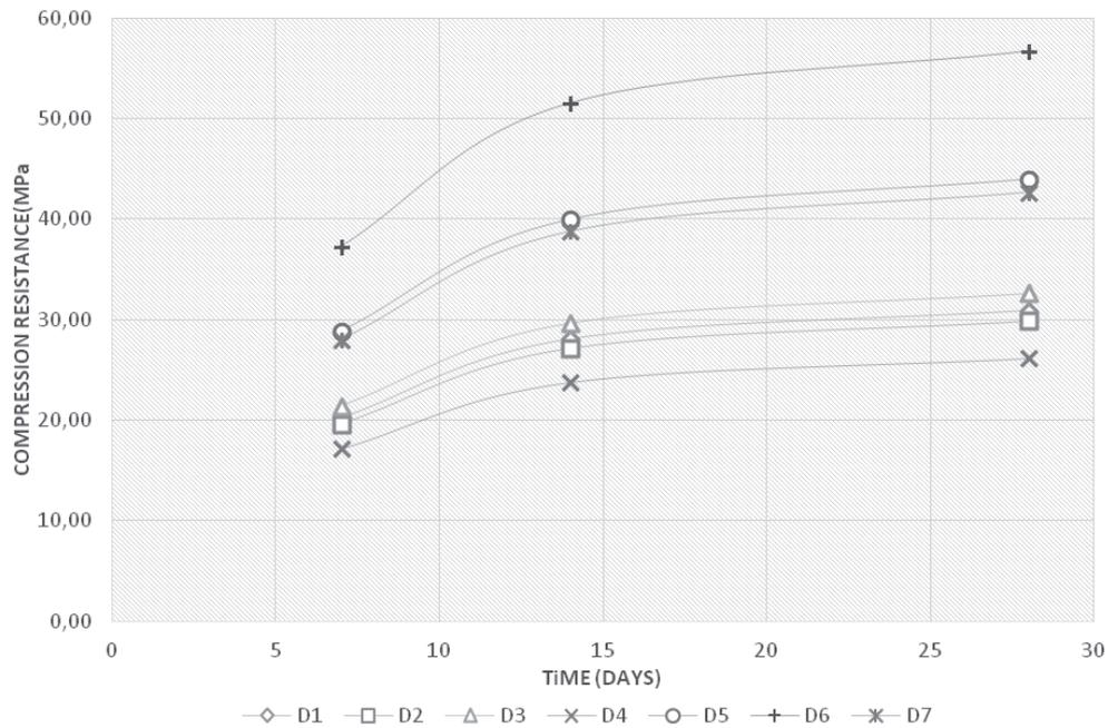
FIGURE 3. Evolution of the long-term compressive strength
