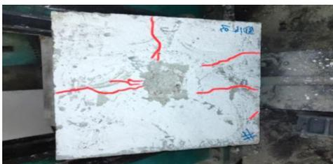
FIGURE 23. Failure mode of specimen with t18 and one layer of geogrid at 5 cm
