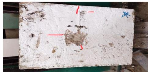
FIGURE 24. Failure mode of specimen with t18 and two layers of geogrid at 5 cm
