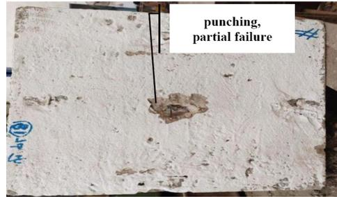
FIGURE 16. Failure pattern of 15 cm slabs with two layers of geogrid at 5 cm after impact loading
