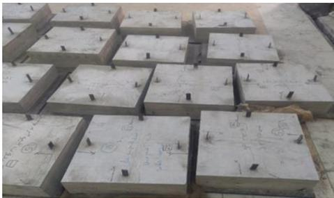
FIGURE 2. Labeled RC samples after unmolding
