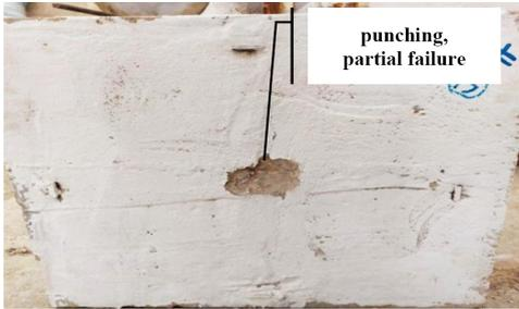
FIGURE 15. Failure pattern of 18 cm slabs with two layers of geogrid at 3 cm after impact loading
