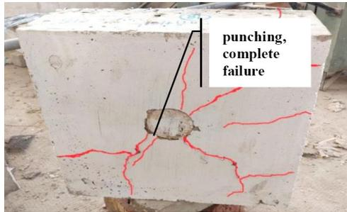
FIGURE 12. Failure mode of control specimen t18 with one-layer geogrid under static loads only
