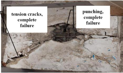
FIGURE 13. Failure pattern of 12 cm slabs with two layers of geogrid at 3 cm after impact loading
