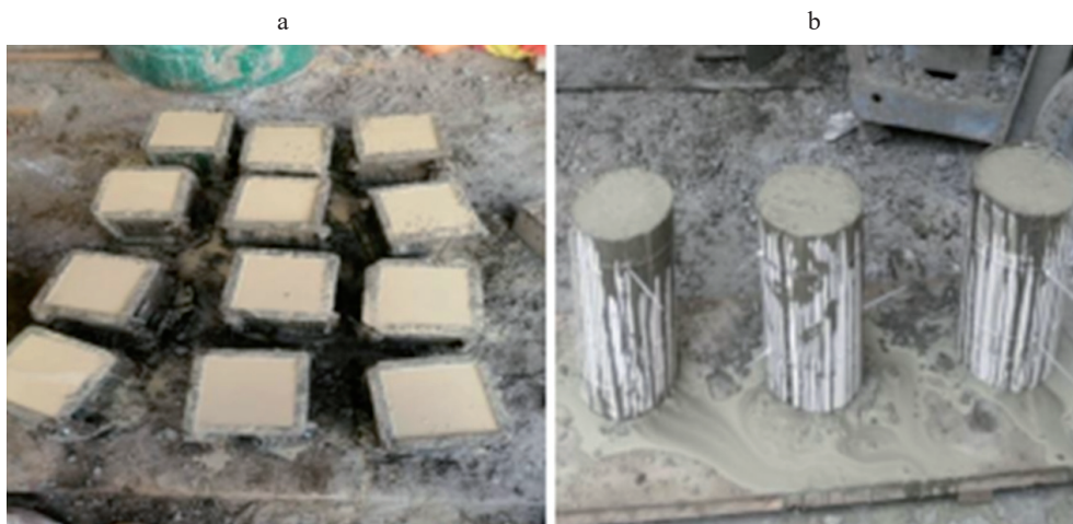
FIGURE 1. The cubic (a) and cylindrical (b) specimens in the molds
