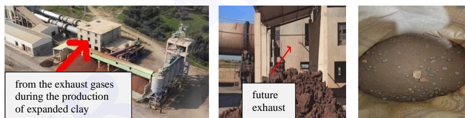
Figure 2. Source of expanded clay kiln dust (ECKD) raw material
