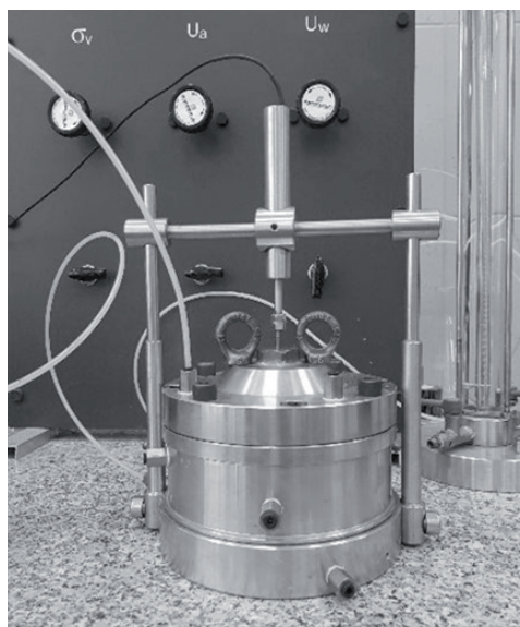
FIGURE 5. Consolidometer used in tests
