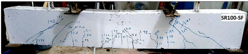
FIGURE 12. Crack pattern of SR100-SF
