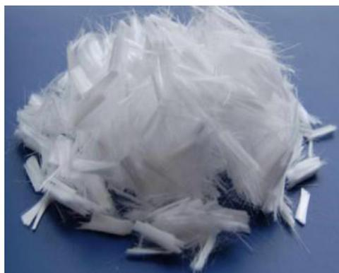
FIGURE 2. Used polypropylene fiber
