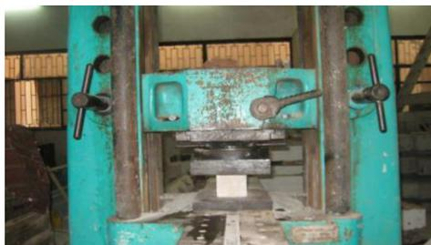
FIGURE 3. Compressive strength test
