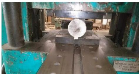
FIGURE 4. Indirect tensile strength test
