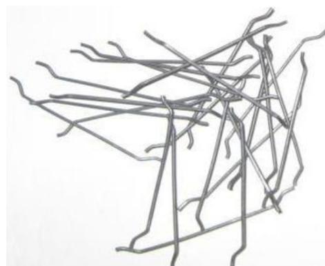
FIGURE 1. Used steel fiber
