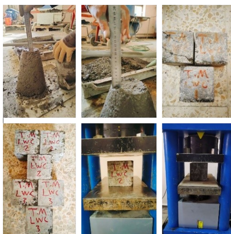
FIGURE 5. Some trial mixes and their compression tests
