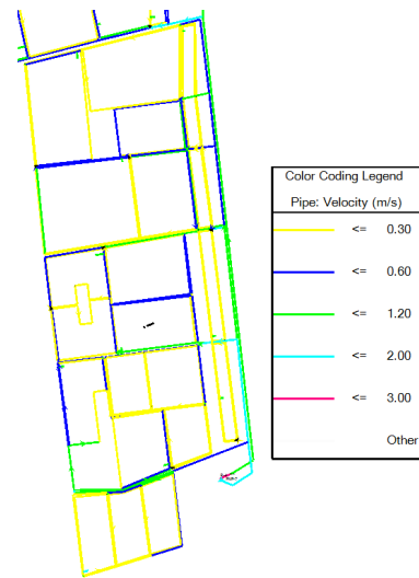
FIGURE 12. The ranges of velocities in the water distribution system at minimum water demand
