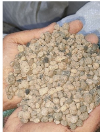
FIGURE 2. Shows lightweight expanded clay aggregate (LECA) used in the current study
