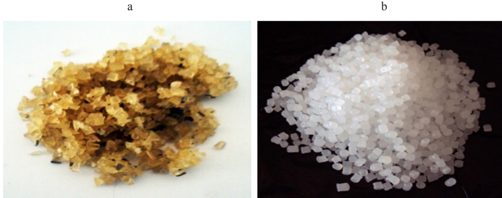
FIGURE 1. Styrene butadiene rubber SBR1502 (a) and low-density polyethylene (b)
