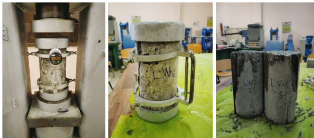
FIGURE 10. Modulus of elasticity test and mode of failure for samples
