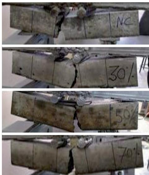
FIGURE 8. Fracture position in concrete prisms
