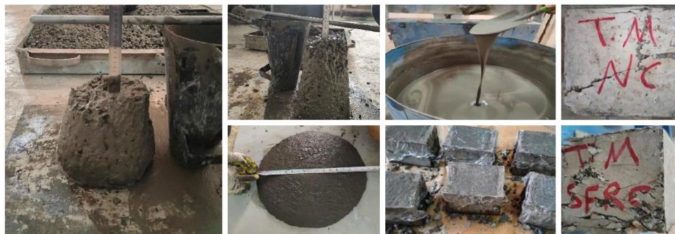
FIGURE 3. Trail mix and fresh concrete test
