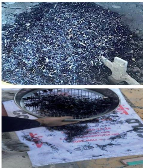
FIGURE 1. Technique for processing recycled steel fibre
