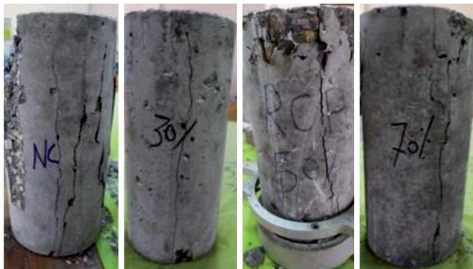
FIGURE 7. Cylinders failure mode
