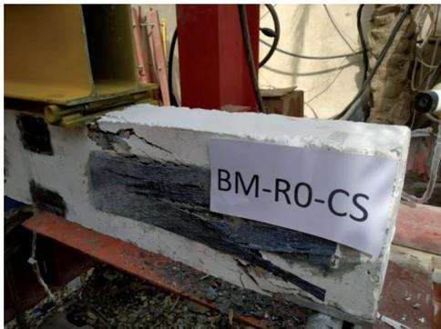
FIGURE 8. Modes of failure of beam BM-R0-CS
