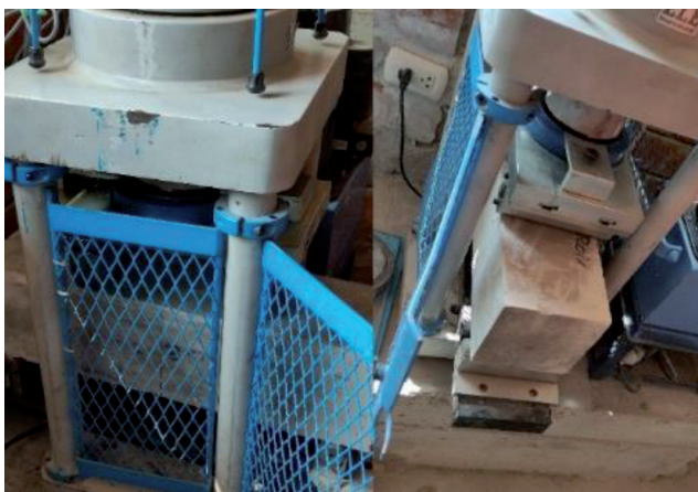
FIGURE 4. Flexural strength concrete test
