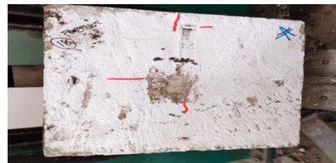
FIGURE 24. Failure mode of specimen with t18 and two layers of geogrid at 5 cm Source: own work.
