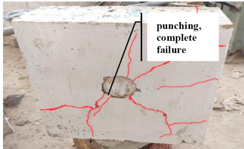
FIGURE 12. Failure mode of control specimen t18 with one-layer geogrid under static loads only Source: own work.
