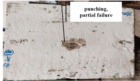
FIGURE 16. Failure pattern of 15 cm slabs with two layers of geogrid at 5 cm after impact loading Source: own work.
