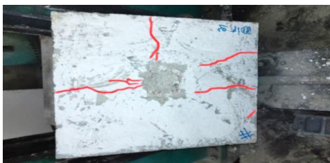
FIGURE 23. Failure mode of specimen with t18 and one layer of geogrid at 5 cm Source: own work.
