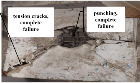
FIGURE 13. Failure pattern of 12 cm slabs with two layers of geogrid at 3 cm after impact loading Source: own work.
