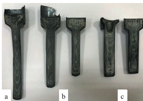
FIGURE 6. Image of samples with a coordinate grid applied after the hot extrusion process: a – for a sample with a final diameter of 10 mm; b – for samples with a final diameter of 12 mm; c – for samples with a final diameter of 14 mm
