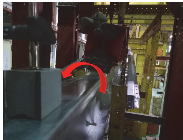
FIGURE 10. Lateral-torsional buckling of the beam
