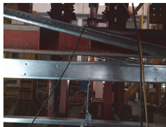
FIGURE 11. Crushing failure on the beam's top flange
