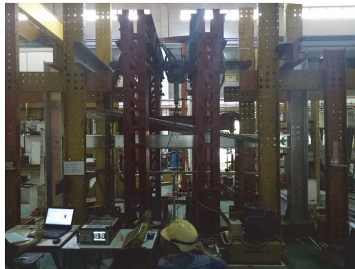
FIGURE 7. Full-scale test using the sub-assembly frame test method
