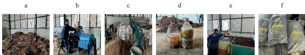
FIGURE 8. Circular resource system: (a) collection of organic waste (leaves) in campus areas, (b) staff conducting the grinding of organic waste, (c) results of the grinding process, (d) biomol production process for compost decomposition bacteria, (e) ground organic waste periodically watered with the biomol solution, and (f) organic compost products ready for use or marketing
