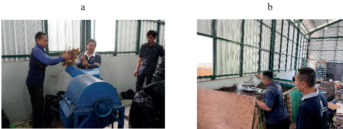
FIGURE 3. Campus waste management system: (a) organic waste shredding; (b) compost fermentation Source: own field documentation (2025).
